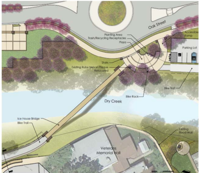
Rotation of the Rube Nelson Ice House Bridge and Extension of the Class I Trail
